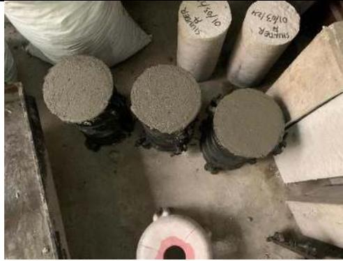
Gambar 1. Uji Silinder 150 x 300 mm
