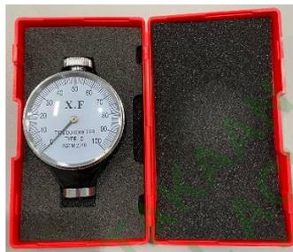
**Gambar 3.4 Shore D Hardness Tester (Durometer)**
